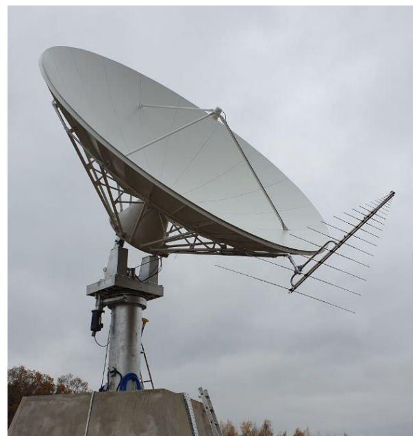
6m antenna with side LPDA to cover low frequency band 100MHz to 1 GHz and wideband feed of 1 to 6 GHz Note: this mount is Normal SRT60 and not SRT60-Pro
