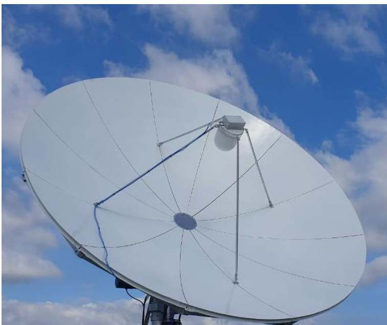
3.7m antenna with 1GHz to 6GHz wideband feed
