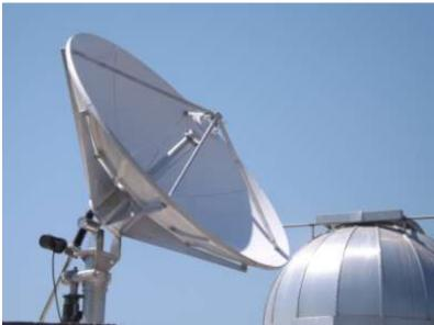
RTP30 consists of 8-panel 3.0 meter dual reflector dish with Az over El pedestal configuration. The pedestal is mounted on a rigid base extension tube suitable for installation on ground or rooftop with an optional NPM (None penetrating Mount).
